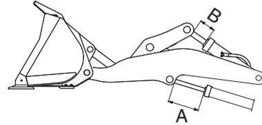
A : Retraction of boom cylinder rod
