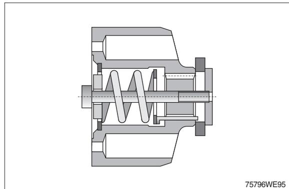
(5) Assemble piston with retaining plate.
